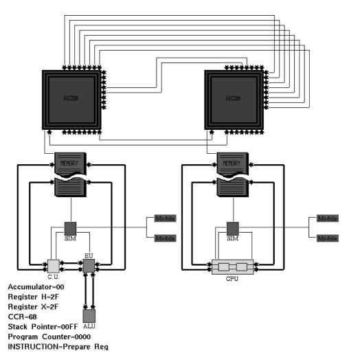
Figure 3: Two M68HC08 micro controllers
