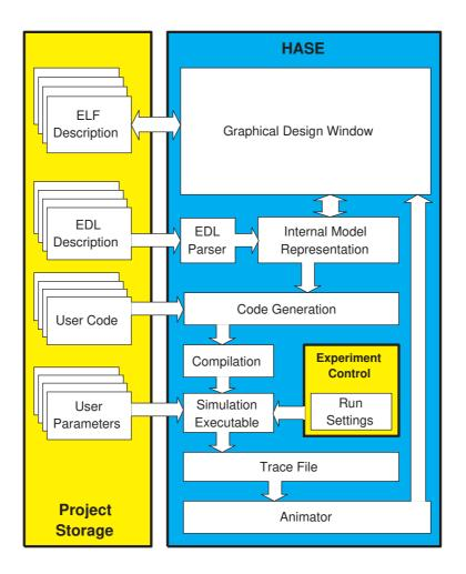
Figure 1: HASE Software Architecture
